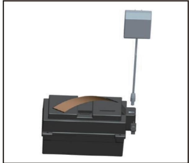
2. Take out the battery. Charge the battery independently.
